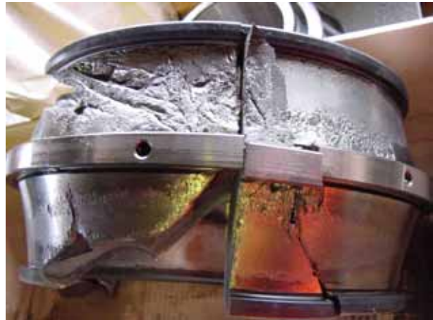
Figure 19: Cracked inner ring of a spherical roller bearing
