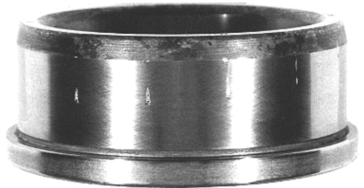
Figure 24: Score marks in the raceway of a cylindrical roller bearing inner ring caused by out-of-square insertion into the rolling element set
