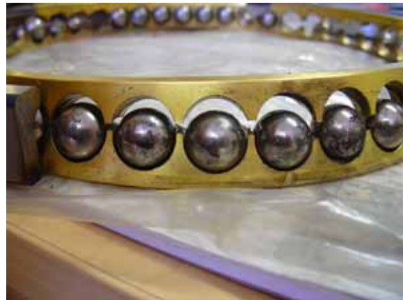
Figure 28: Cage split in half due to lubrication starvation at high speed
