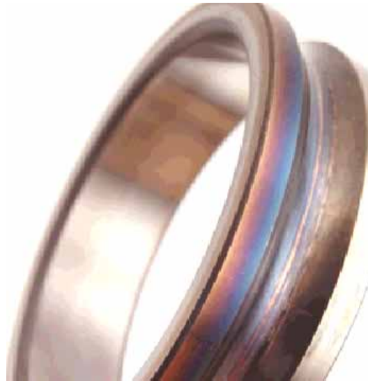
Figure 25: Colour changes and deformations of the raceway due to extreme temperatures
