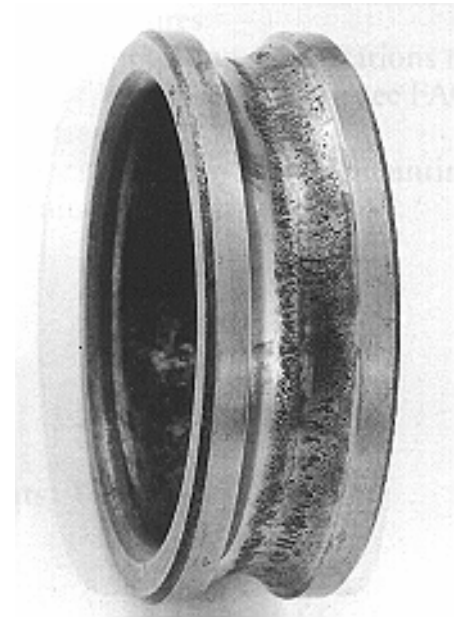
Figure 4 Deep groove ball bearing with tracks due to contamination in bearing or lubrication
