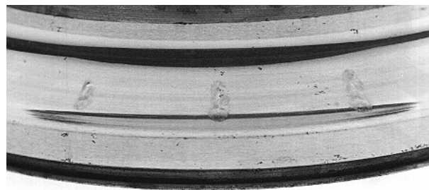
Figure 15: False brinelling marks on the inner ring of an angular contact ball bearing
