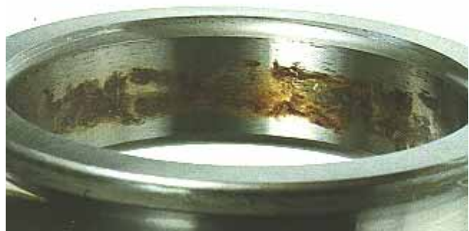
Figure 2: Fretting corrosion reveals the size of the load zone at the stationary outer ring
