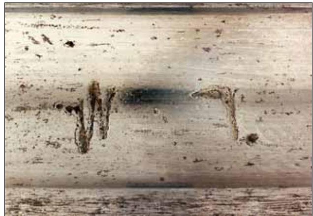
Figure 18: Fusion Crater on the inner ring raceway of a cylindrical roller bearing due to welding
